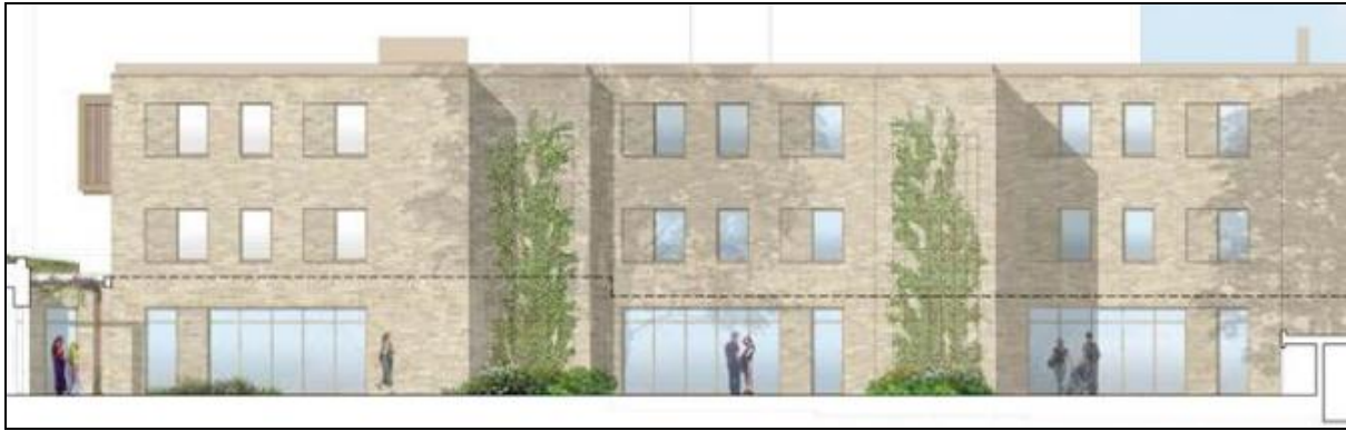
Fig. 19: Rear elevation of the proposed building showing large windows/doors at ground floor level helping to link inside and outside areas. This improved ground floor detail is in response to DRP comments.
