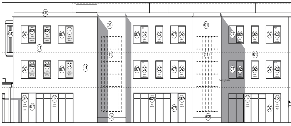
Fig. 30: Showing window detail and glazing to proposed rear elevation. Windows annotated with the number 02 would have either clear glazing or white translucent glazing. Openings annotated with the number 07 would be recessed brick panel.
